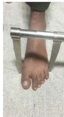
Fig. 2: Measurement of foot breadth
