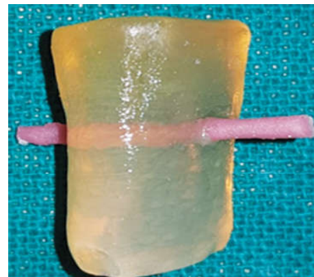
Fig. 7: Customised glycerine soap bolus with cold cure stabilizing rod.
