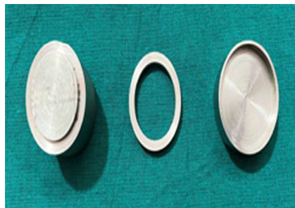
Fig. 2: Stainless steel mold measuring 1.5 mm x 50 mm
