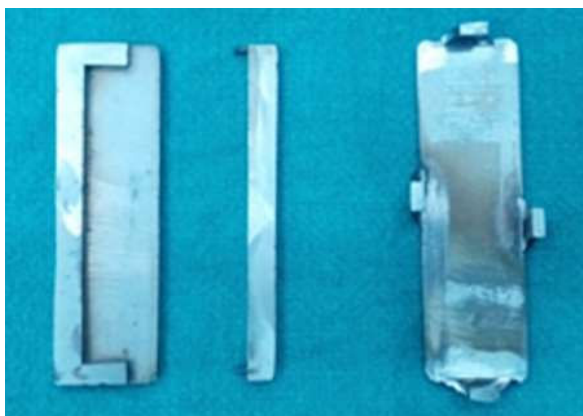
Fig. 1: Stainless steel mold measuring 65mm x 10mm x 2.5mm
