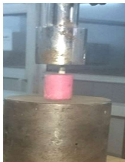
Fig. 7: Pull- off test on UTM
