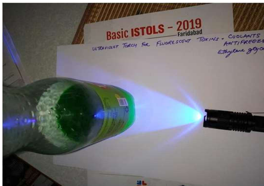
Fig. 9: Ultraviolet fluorescence of Car AC coolant- ethylene glycol- toxic alcohol (glows in UV torch) for on-spot diagnosis Last year, we have conducted ISTOLS on 24th-25th June 2018 in Medanta-the Medicity successfully by training 21 resident doctors, NRHM Rural Medical Officers of Haryana and consultants in critical care, emergency, forensic medicine and toxicology. Last year, we have conducted ISTOLS course on 24th-25th June 2018 in Medanta-the Medicity successfully by training 21 resident doctors, NRHM Rural Medical Officers (RMO) of Haryana, Rajasthan and Delhi NCR consultants in critical care, emergency, forensic medicine and toxicology.
