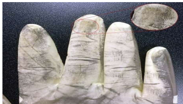
Fig. 7: Latex gloves treated with Cyanoacrylate method.
