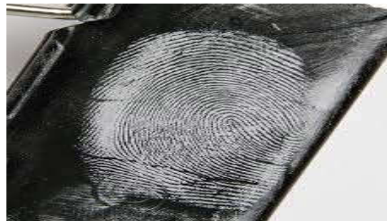
Fig. 4: Magnetic powder on a piece of latex gloves
