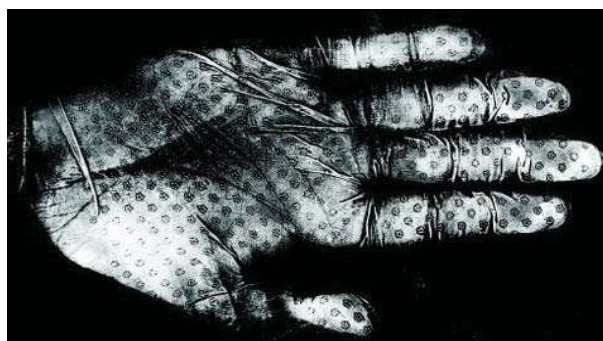
Fig 8: Latex gloves treated with iodine fuming method
