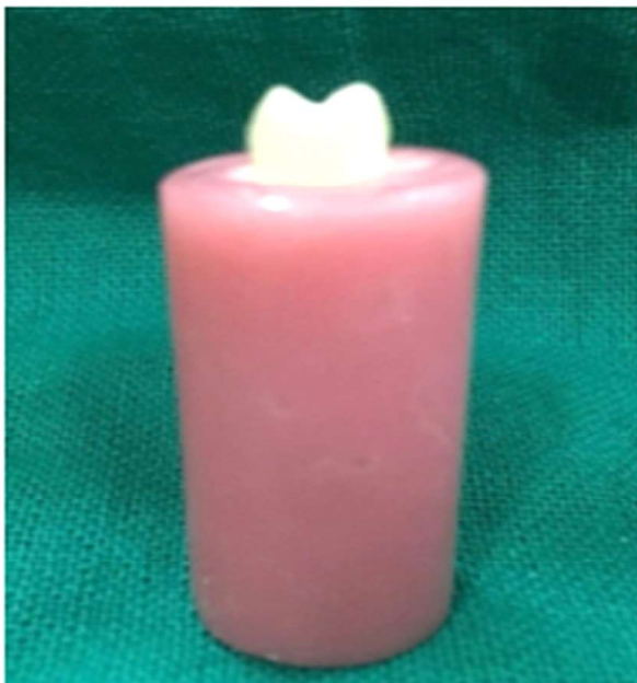
Fig. 2: Tooth embedded in acrylic block
