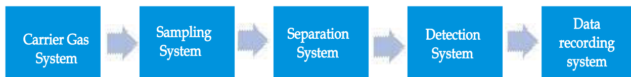
Fig. 4: Parts of a basic Chromatographic system.
