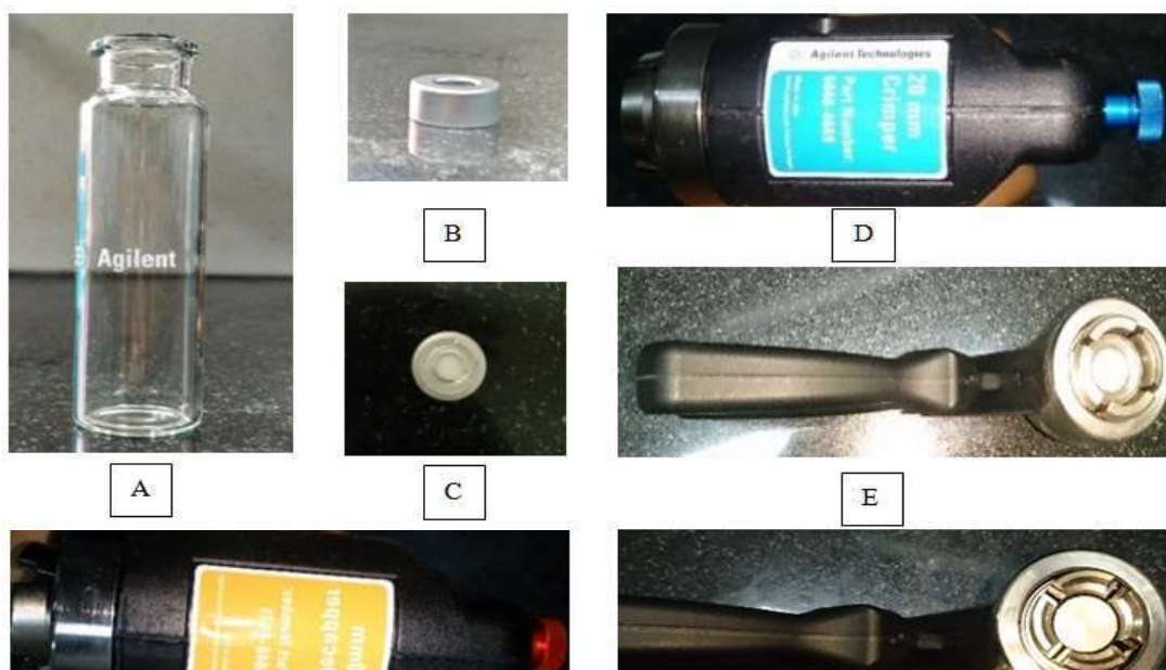
Fig. 10: Accessories of Gas Chromatography Headspace: A) 20ml GC-HS Vial, B) Metallic Crimp, C) PTFE Septa, D) Top View Crimper, E) Bottom view Crimper, F) Top View Decrimper, G) Bottom view Decrimper (Image source: Toxicology Lab, Dept of FMT, AIIMS).
