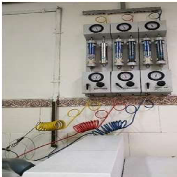
Fig. 5: Gas traps for introduction of Nitrogen, Zero Air and Hydrogen in GC System (Image Source: Toxicology Lab, Dept of FMT, AIIMS).
