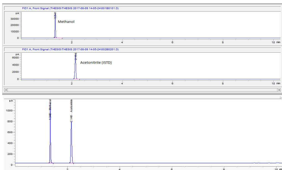
Fig. 13: Chromatogram showing acetonitrile, standard methanol, methanol standard and mixture of standard and internal standard in the matrix (Image source: Toxicology lab, Deptt of FMT, AIIMS).
