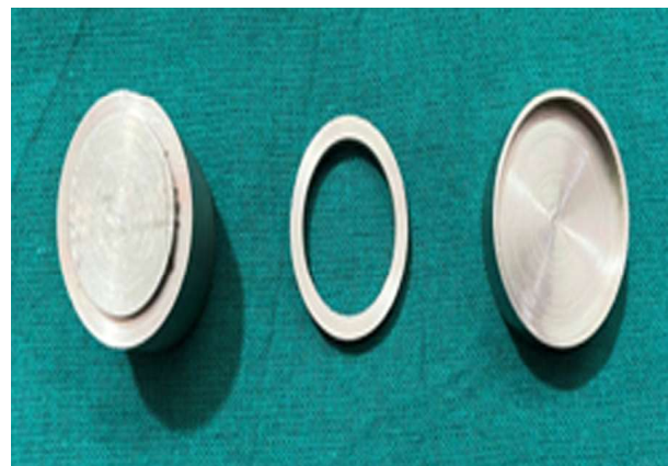
Fig. 2: Stainless steel mold measuring 1.5 mm x 50 mm
