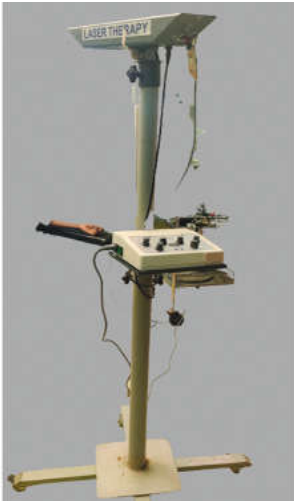
Fig. 2: Gallium arsenide (gas) diode red laser used for Low level laser therapy.
