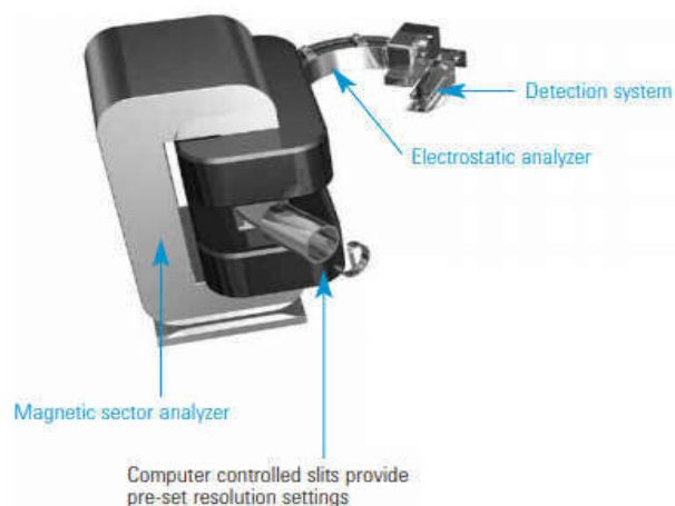
Fig. 9: Schematic of Magnetic Sector Analyzer.
