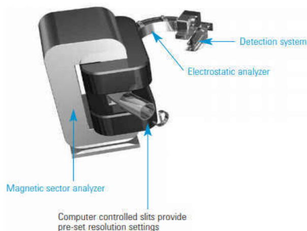
Fig. 9: Schematic of Magnetic Sector Analyzer.
