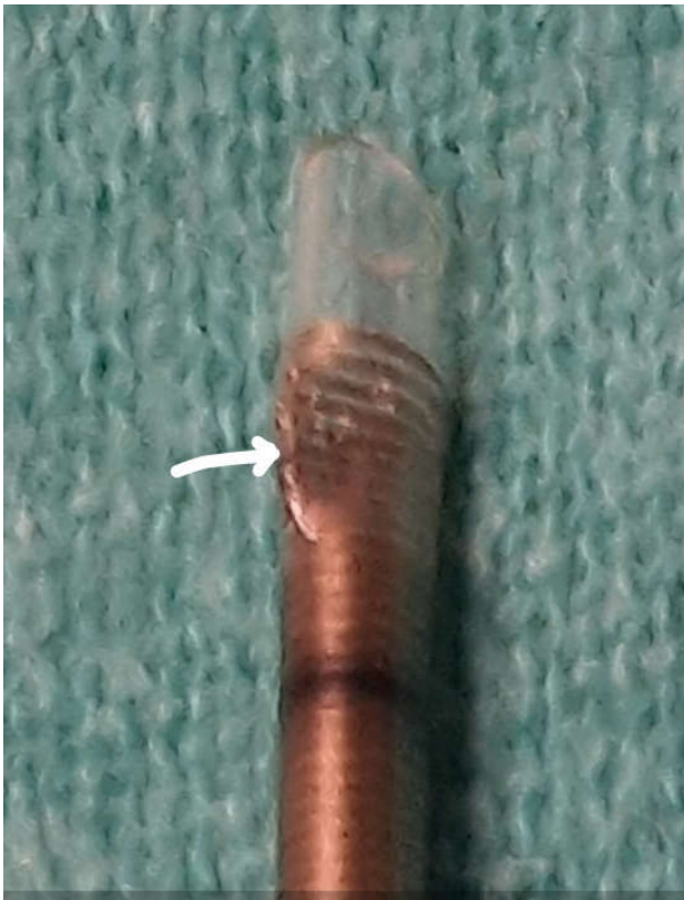
Fig. 1: Image showing the compression (indicated by white arrow) of aortic cannula due to breakage of reinforced wire inside the lumen wall.
