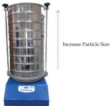
Fig. 1: A set of sieves mounted on a shaker for straining soil
