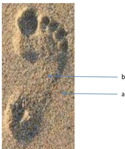
Fig. 3: Control soil samples need be collected from (a) just outside the impression and (b) from within the impression.
