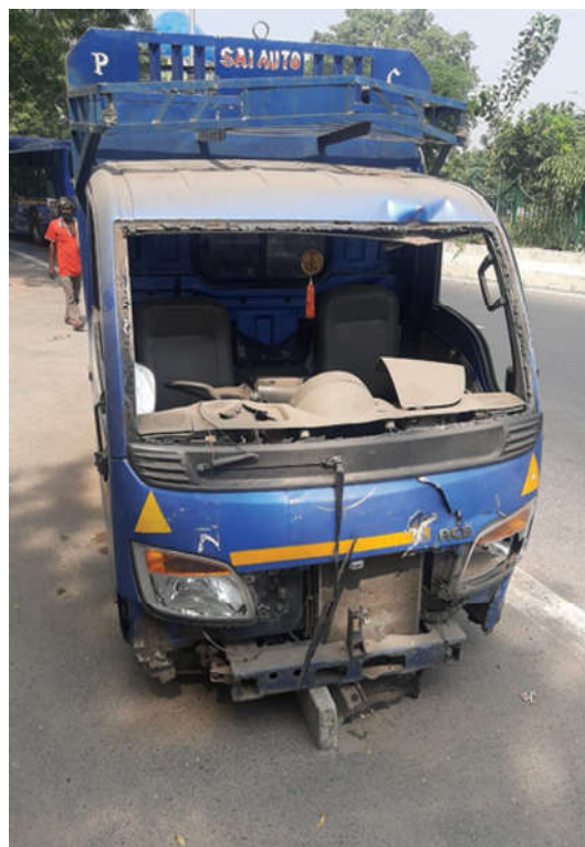
Fig. 6: Damaged front of mini truck.
