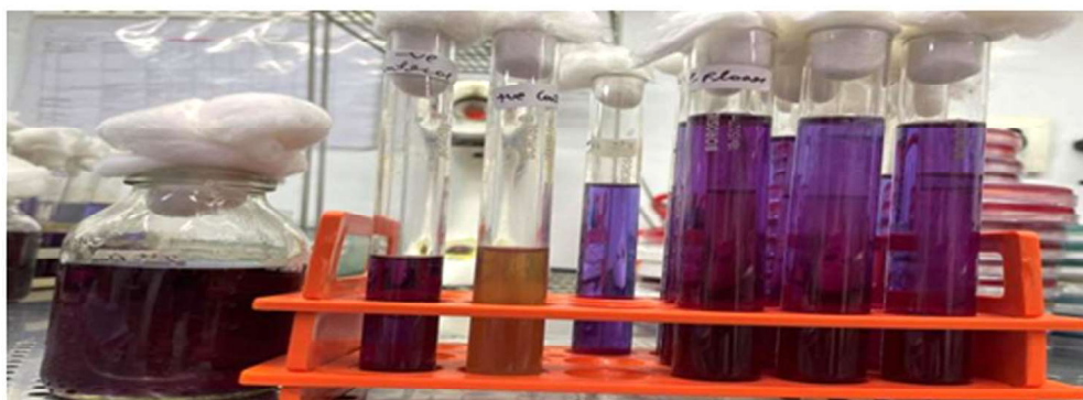
Fig. 1: Multiple Tube Test using MacConkey broth Purple (MCBP) (double strength) with Bromocresol purple (BCP) with positive and negative controls
