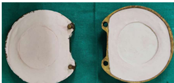
Fig. 4: Mold space after dewaxing
