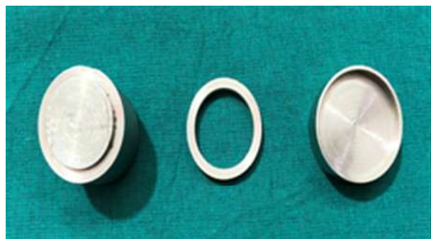
Fig. 1: Stainless steel Die (1.5 mm x 50 mm)
