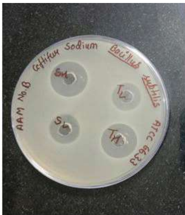
Fig. 2: Two level agar diffusion assay method using a test microorganism Bacillus subtilis ATCC-6633 (MTCC 441) at concentration of Reference solution S_H = 4 \mu\text{g mL}^{-1} , S_L = 1 \mu\text{g mL}^{-1} and Sample solution S_H = 4 \mu\text{g mL}^{-1} , S_L = 1 \mu\text{g mL}^{-1} .
