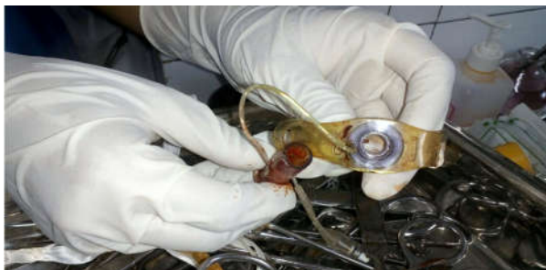
Fig. 4: Clean cut break at the flange and tube junction suggestive of manufacturing flaw
